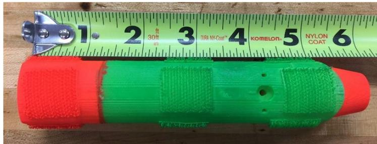
Note: The "Injector" measures 6 inches long, 1 1/16 inches thick/tall and 1 3/8 inches wide. Competitors must devise a method to carry and release the "injector". Weight = 45g to 55g
