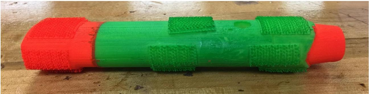
**Note: The "Injector" measures 6 inches long, 1 1/16 inches thick/tall and 1 3/8 inches wide. Competitors must devise a method to carry and release the "injector". Weight = 45g to 55g**
